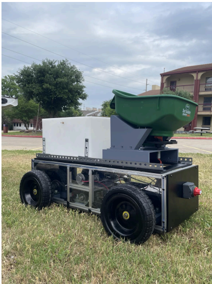
Figure 1: Final Assembly of the Garden Cultivation Robot with Subsystems Attached
