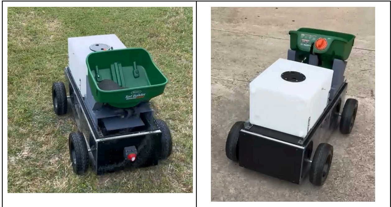
Figure 18: Robot testing on uneven terrain; note fertilizer distribution in spiral pattern and water spray (left), robot testing on hard terrain (right)
