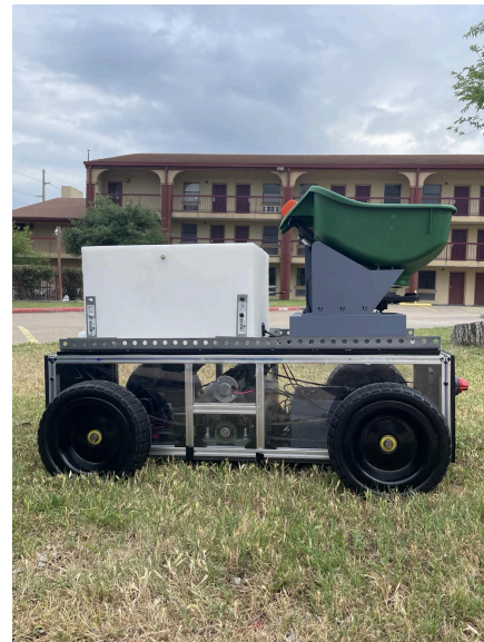
Figure 1: Final Assembly of the Garden Cultivation Robot with Subsystems Attached
