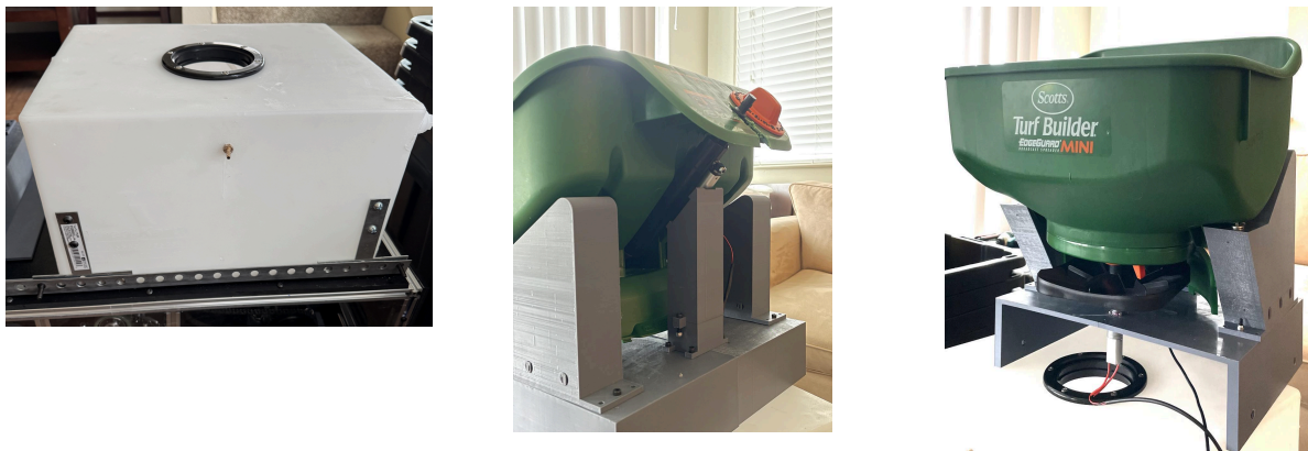
Figure 8: Water subsystem mounted on robot (left), fertilizer base attached to 3D printed platform with linear actuator attached (middle), fertilizer base with motor attached (right)
