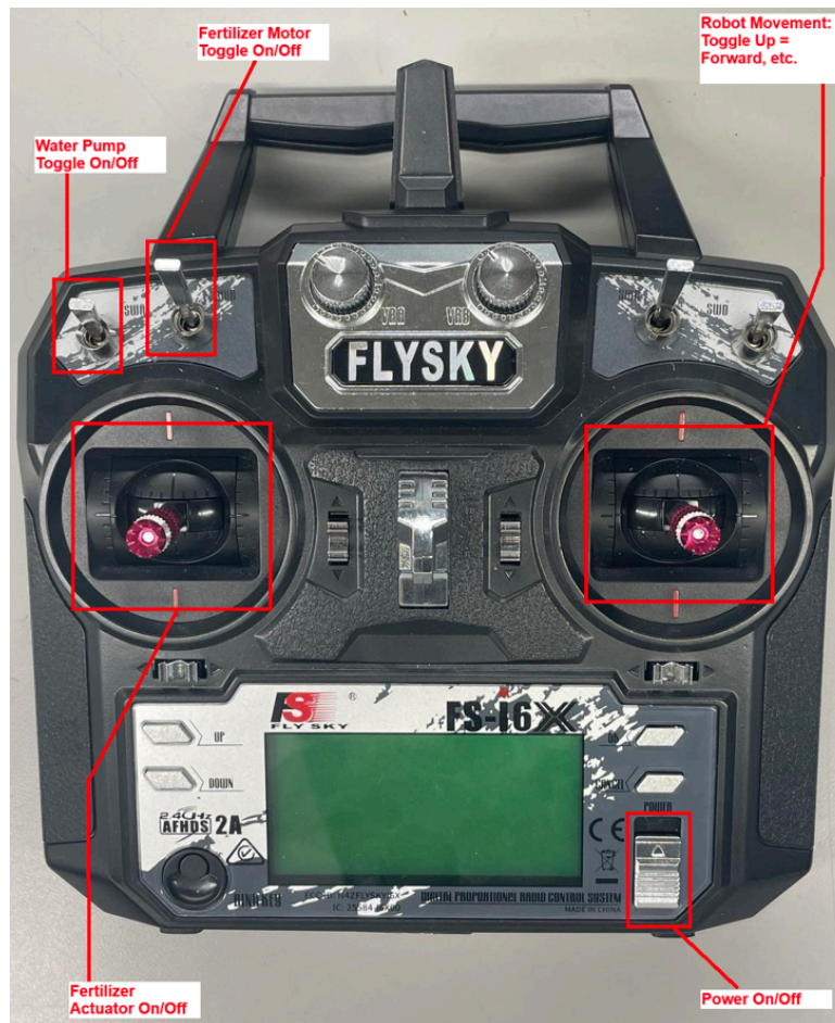
Figure 10: FlySky remote diagram, labeled with robot functions
